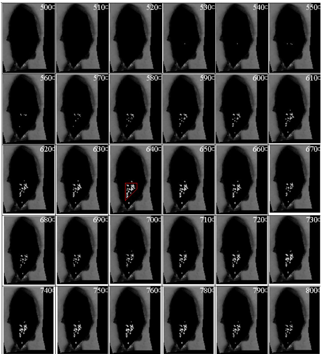
Figure 6: Results of AP1 for the selected ROIL for each wavelength layer (from 500 to 800nm, on the top right of each image) with white pixels reported as the loadings LV1 contribution exceeding the 90th percentile.
