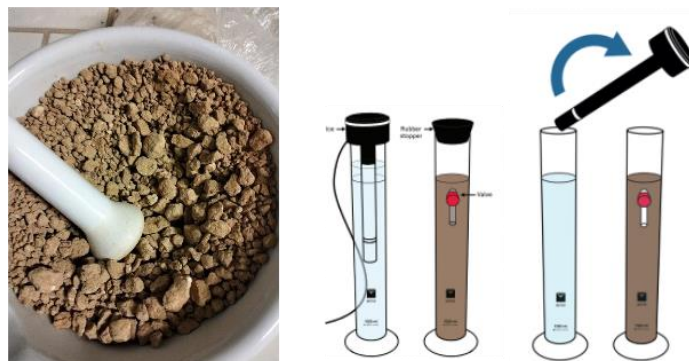
Figure 3.2. Preparation of the sample for analysis in the laboratory mortar (on left), and PARIO Instrument Calibration (on right).
