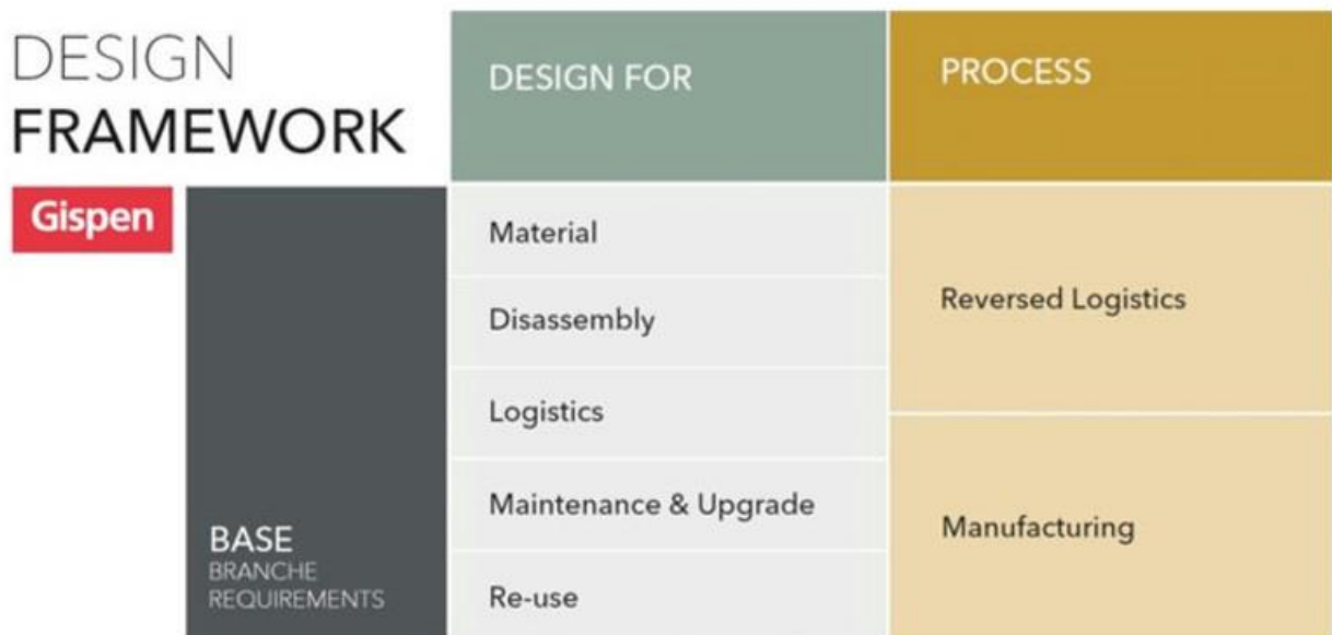
Figura 21 -The Gispén circular economy (CE) design framework Fonte: Bosch, T., Verploegen, K., Grösser, S. N., & van Rhijn, G. (2017). Sustainable furniture that grows with end-users. In Dynamics of Long-Life Assets (pp. 303-326). Springer, Cham.
