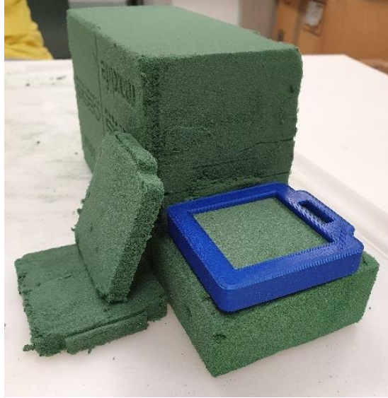
Fig. 3.1.3 Oasis Floral Foam and casting mould of substrate
