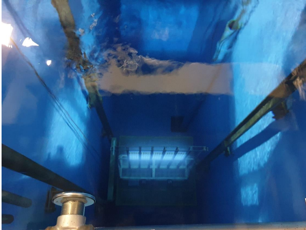
Fig. 1.7.1 ^{60}\text{Co} \gamma irradiation source in BioShield pool
