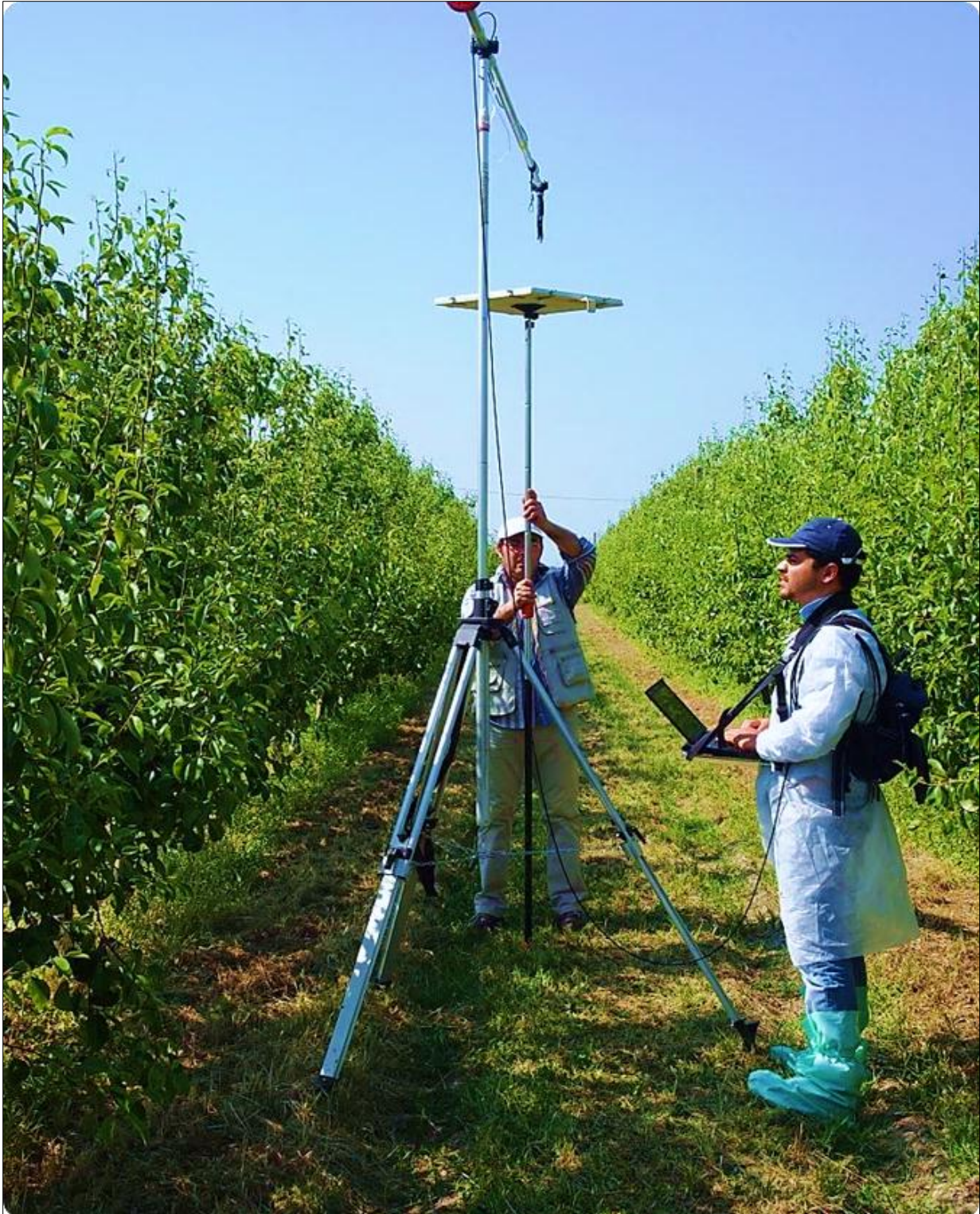
Figure 14 The specially designed tripod that carried the pistol grip to mount the fore-optic above the trees during canopy reflectance measurements.
