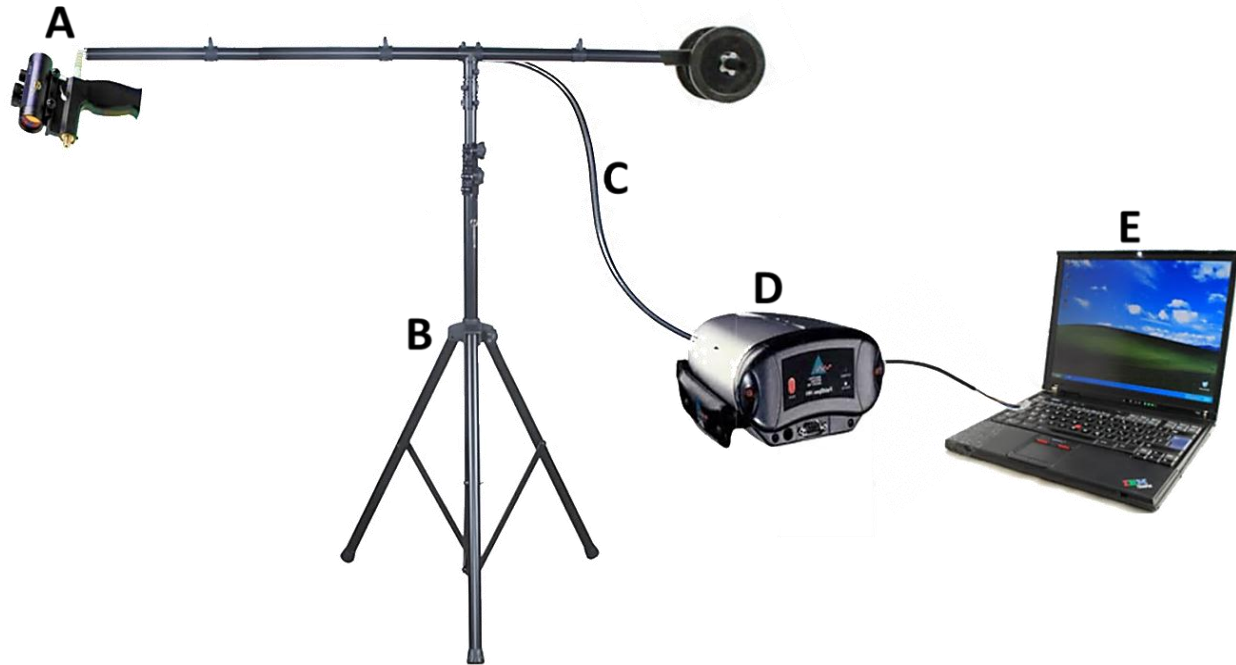
Figure 13 The hyperspectral acquisition system with the supporting system used for canopy reflectance measurements. This system comprised: (A) ASD fore-optic pistol grip, (B) aluminum tripod, (C) optical fiber, (D) ASD FieldSpec® HandHeld2 spectroradiometer, and (E) instrument controller.
