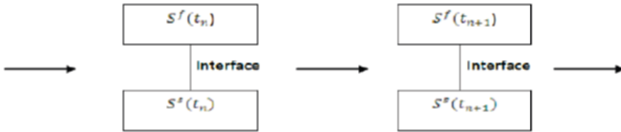
Figure 1.4: Graphical scheme of the partitioned approach. In this approach, the fluid domain equations and the solid domain equations are solved separately one or more times in each timestep and the informations about the congruence are exchanged through the two regions interface.
