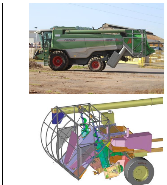
Figure 7. Bionalan back container and schematic representation
