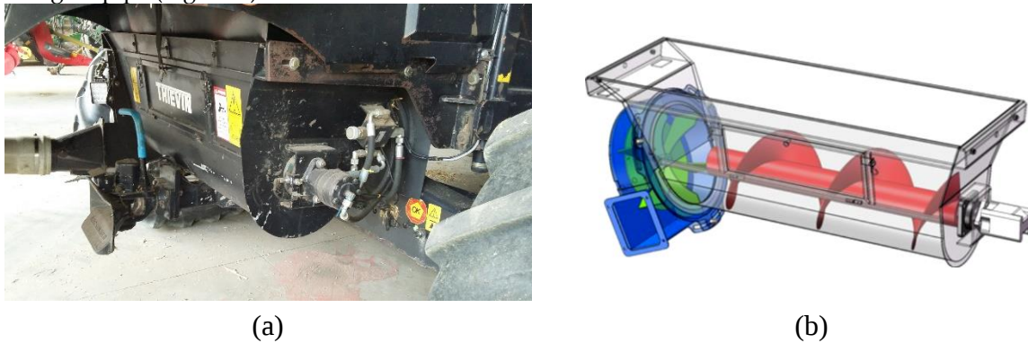
Figure 2. (a) Thievin system “Turbopaille” for chaff collection and (b) schematic representation
