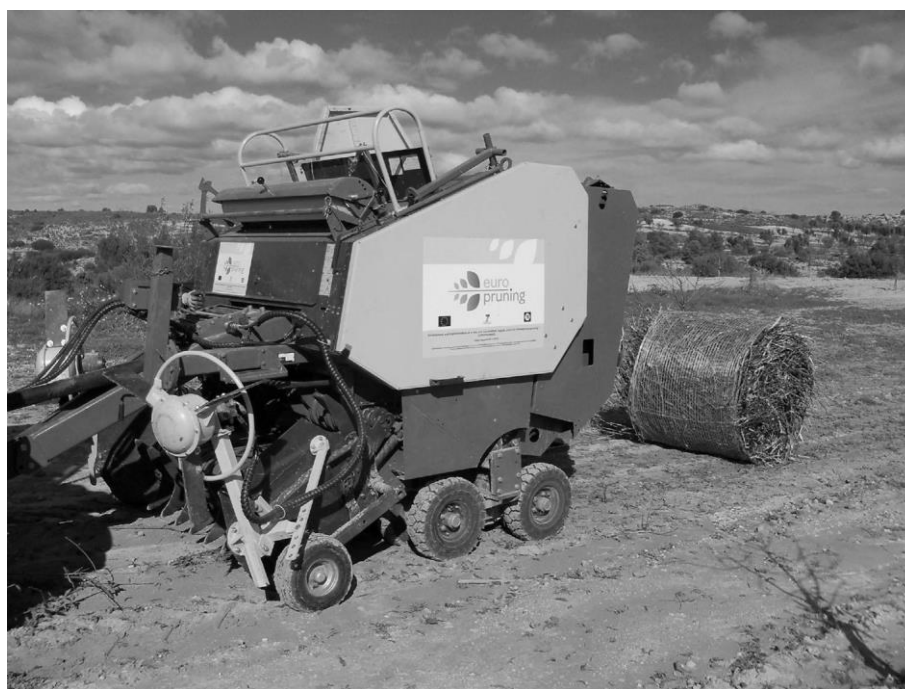
Fig. 3. Innovative pruning baler developed by PIMR (mod. PRB 1,75) during the European project Europruning [23].
