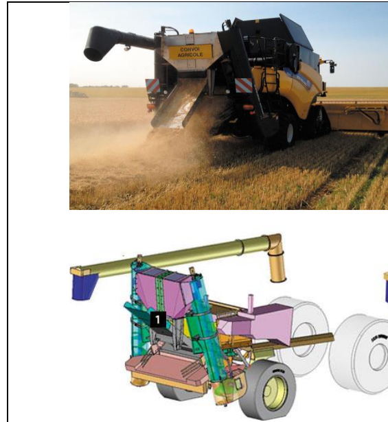
Figure 3. Thierart windrowing system for NH CR combine and schematic representation
