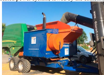
Figure 8. Thierart modular system for continuous pressing of the chaff during threshing
