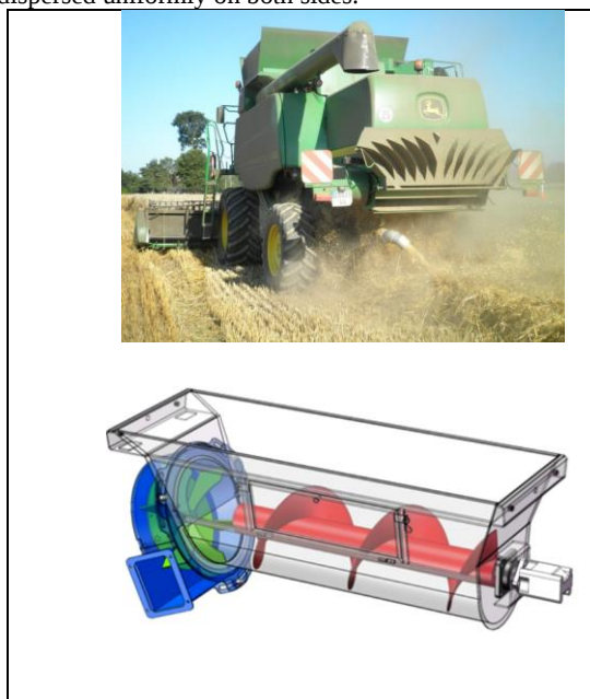
Figure 5. Thievin turbine system with discharge on windrow and schematic representation
