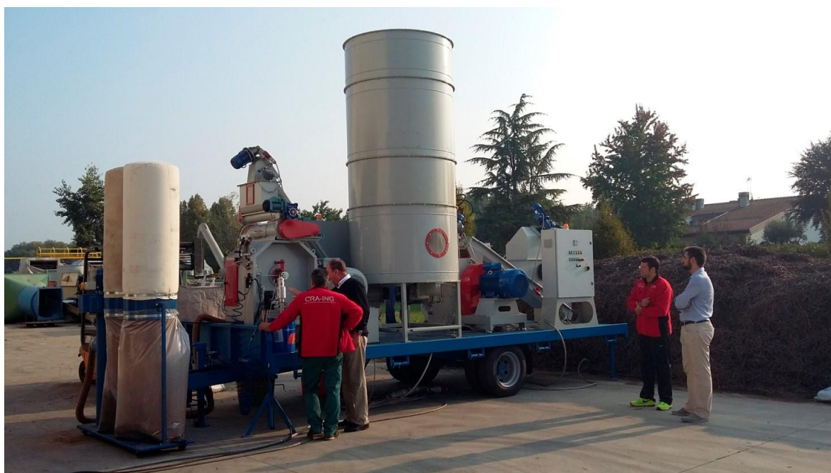
Figure 2. Mobile pelleting plant developed by Costruzioni Nazzareno.
