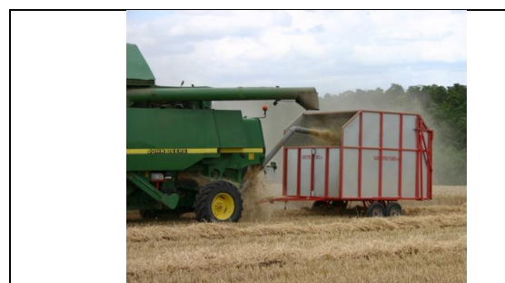
Figure 6. Thievin turbine system with discharge on a trailer towed by a tractor (up) and by the combine itself
