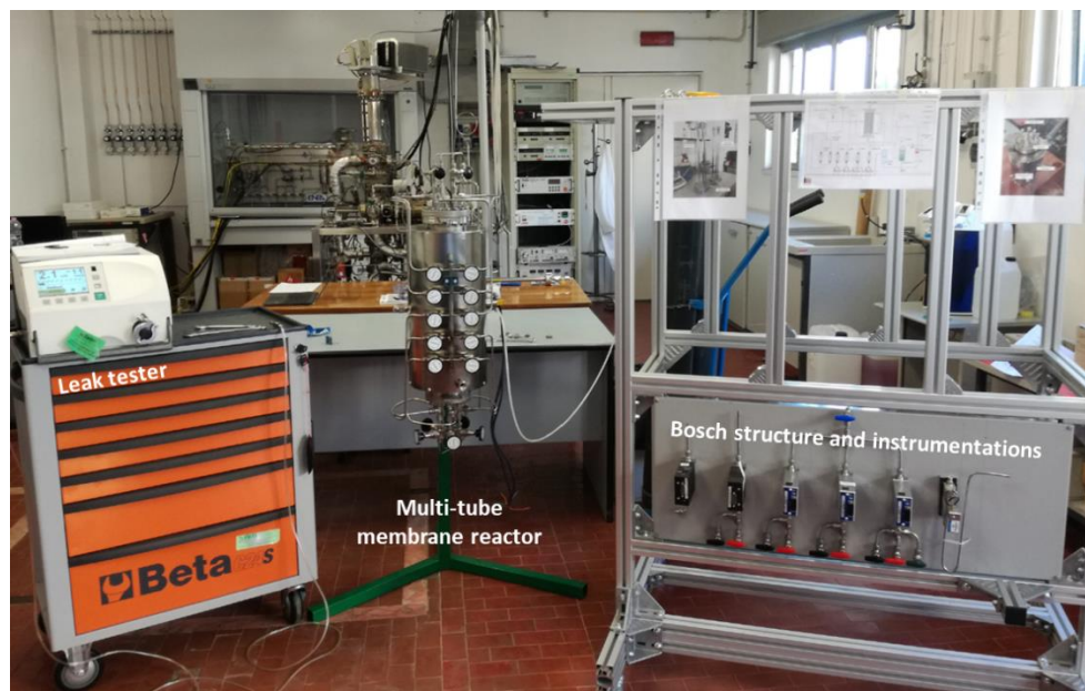
Figure 61. Picture of the MeSMer facility before assembly.
