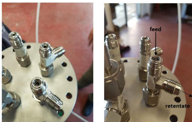
Figure 58. Picture of the Tee-connection attached to each membrane tube.
