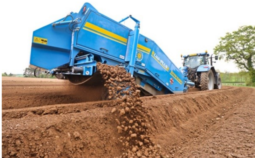
Figure 2.6. Stone separator for windrowed soil.
