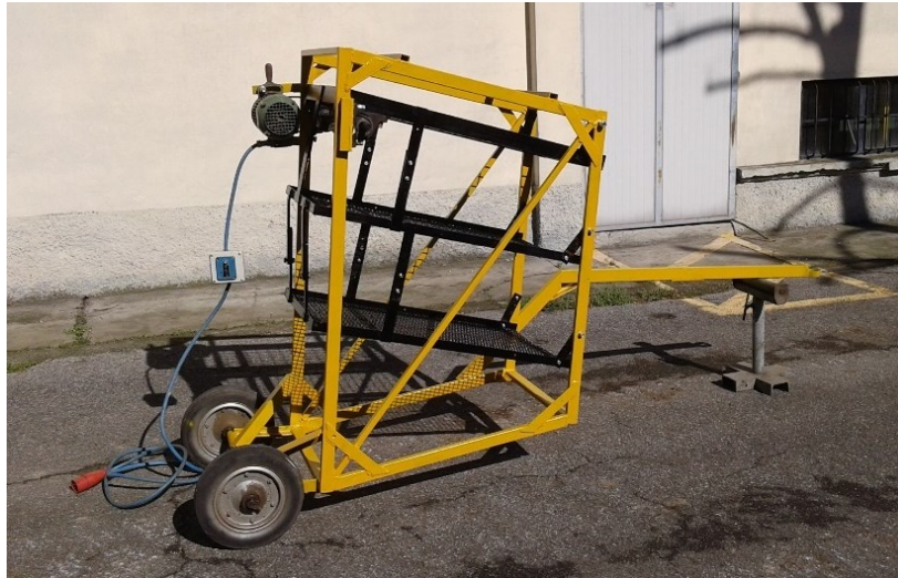
Figure 4.1. The prototype of sieving machine realized.
