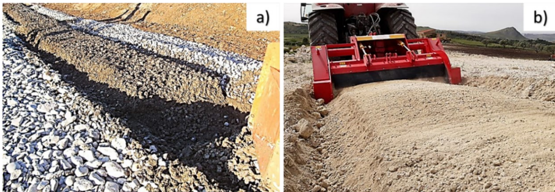
Figure 2.8. a) Crushing efficiency on granite rocks; b) Stone crusher on calcareous rocks.
