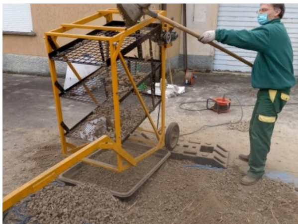
Figure 4.2. Soil screening tests performed at CREA-IT Research Centre with local samples of soil: a) static test; b) dynamic test.
