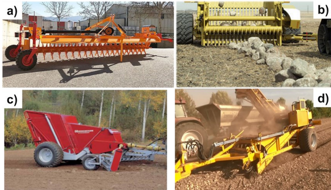
Figure 2.3. Samples of: (a) Stone windrower; (b) Stone picker; (c) Stone windrower & picker; (d) Stone collector with conveyor belt.
