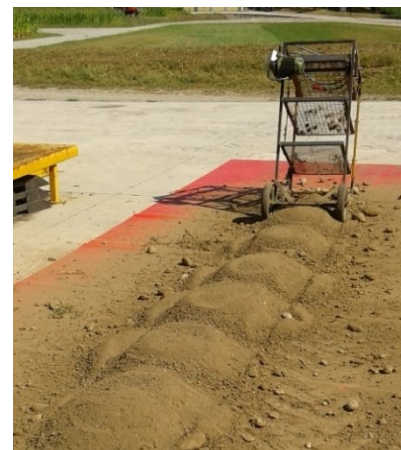
Figure 4.2. Soil screening tests performed at CREA-IT Research Centre with local samples of soil: a) static test; b) dynamic test.
