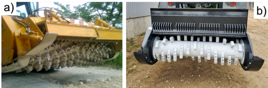
Figure 2.7. a) Stone crusher with teeth for calcareous rocks and b) with hammers for granite rocks.
