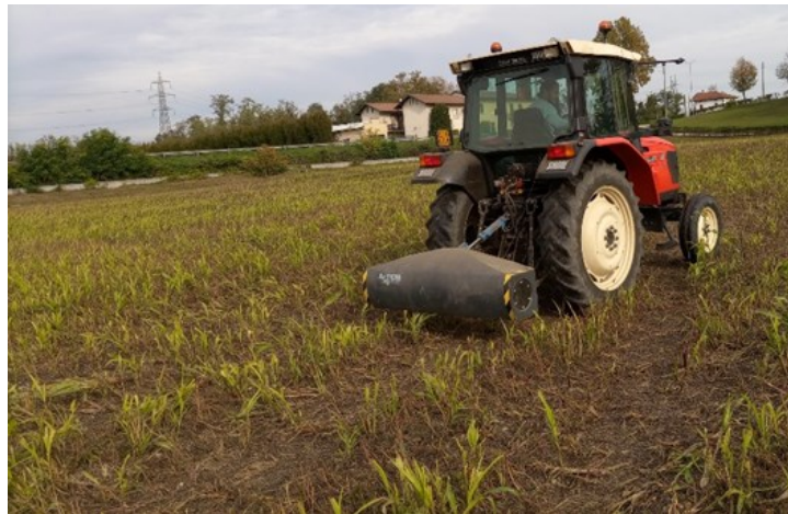
Figure 5.13. The SoilXplorer sensor rear-mounted on a tractor.
