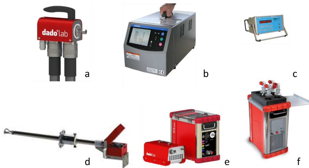
Figure 12 - Instrumentation used for emission sampling during coffee pellet combustion. a) Dadolab HP1 probe, b) Horiba PG250, c) FID Ratfish RS 53-T, d) Dadolab HP5 probe, e) Dadolab Source Tester ST5, f) Dadolab SC5 Smart Chillerha.
