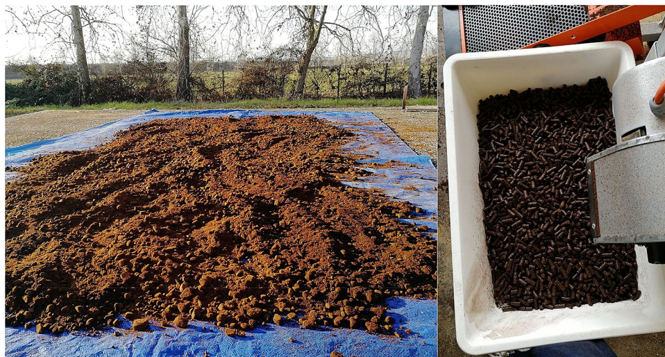
Figure 1. Spent coffee ground (SCG) before (left) and after (right) the pelletizing process.
