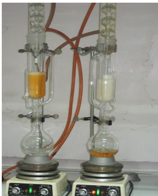
Figure 41. Soxhlet extraction setup used for water and for ethanol extractives determination
