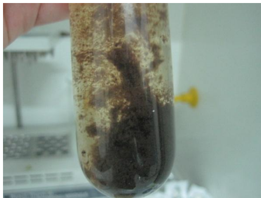
Figure 42. Sample aspect after two-step hydrolysis
