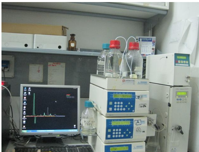
Figure 43. Knauer HPLC system used for fiber analysis
