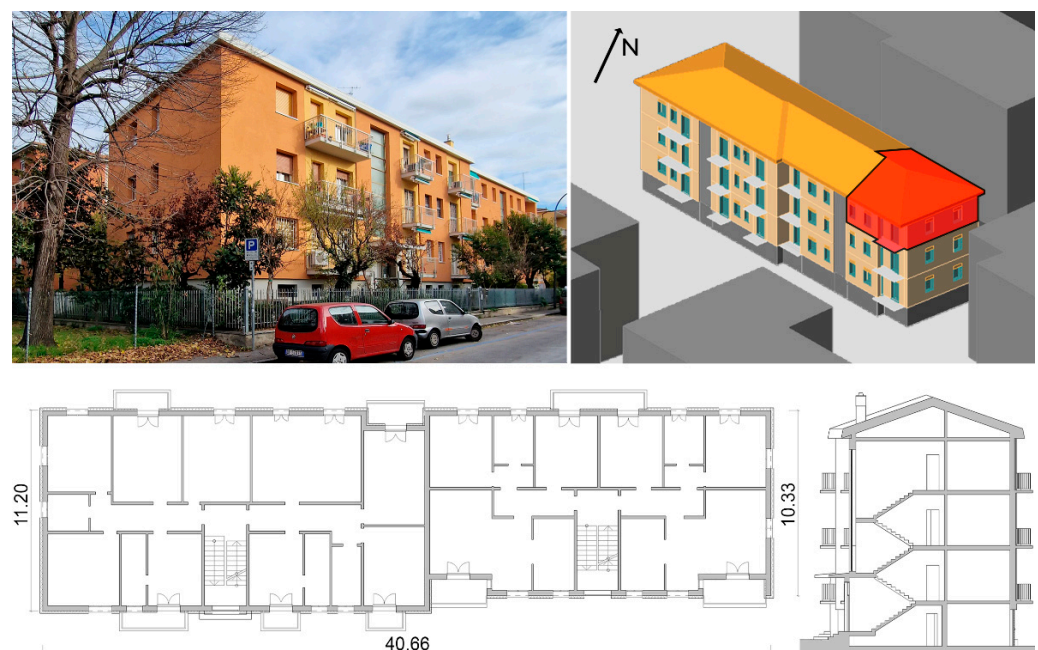
Figure 2. Photograph, typical floor plan, section, and axonometric view of the model with the thermal zone considered for thermal comfort analyses highlighted in red (2024, © Authors).
