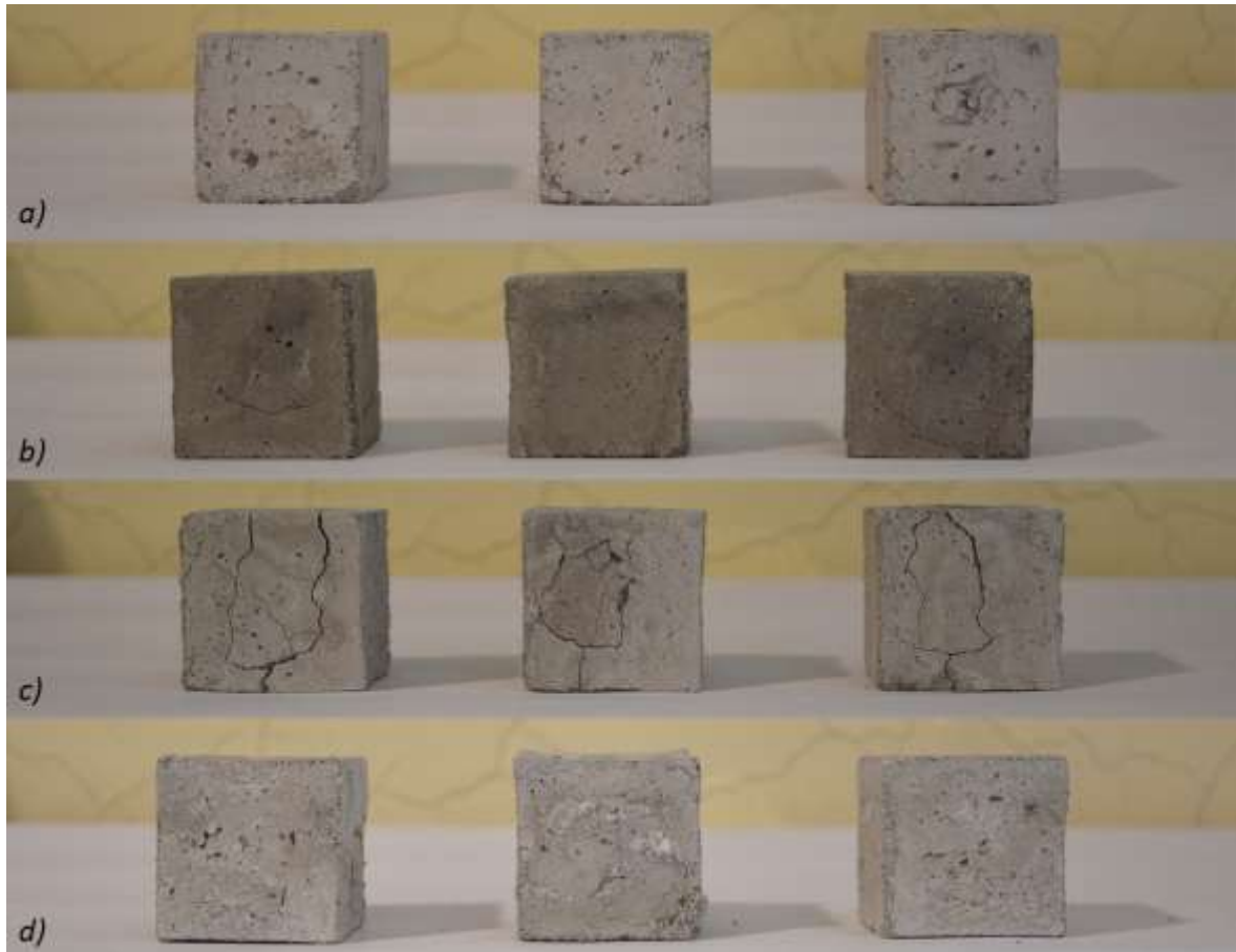
Figure 4.24. Mortar specimens after the ageing treatment: a) specimens exposed to deionized water; b) specimens exposed to sodium chloride aqueous solution; c) specimens exposed to sodium sulphate aqueous solution; d) specimens exposed to potassium nitrate aqueous solution.
