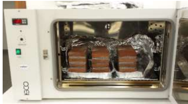
Figure 3.33. Masonry specimens into the oven.
