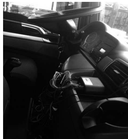
Figure 1. Installing the GPS/GSM black-box unit.
