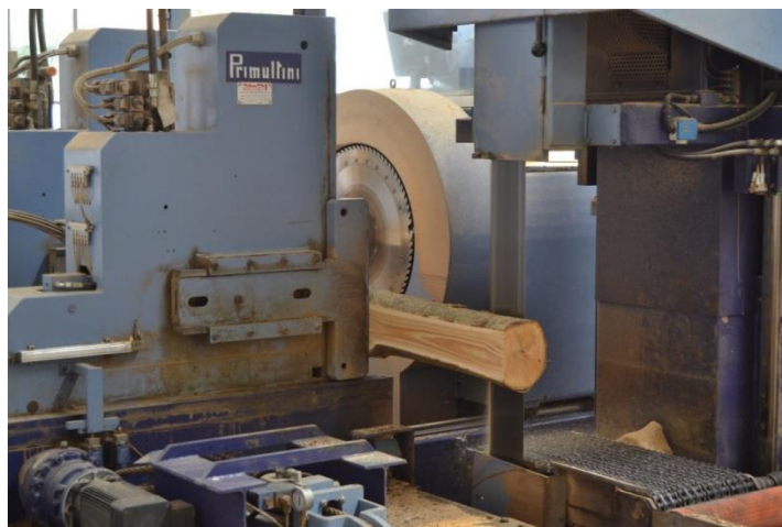
Figure 10 - Determination of thickness with Headsaw
