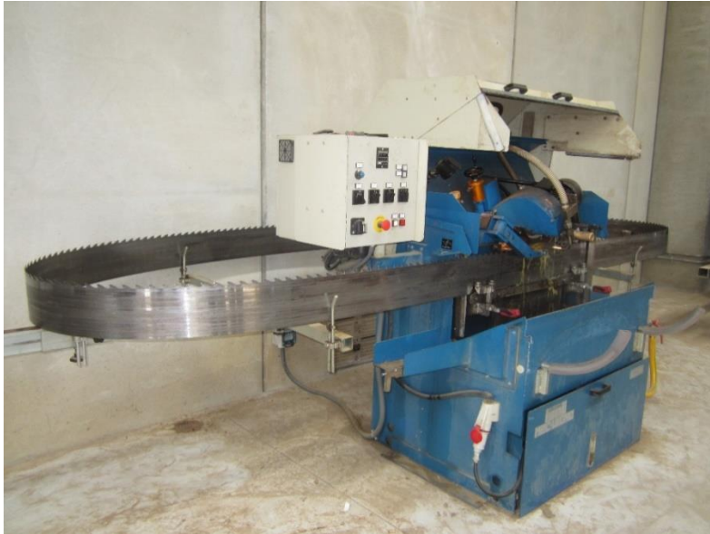
Figure 3 - Blade Sharpening Phase
