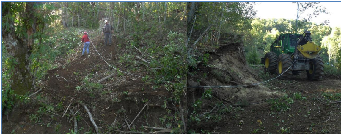
Figure 2- Extracting trees with a John Deere skidder at site A.
