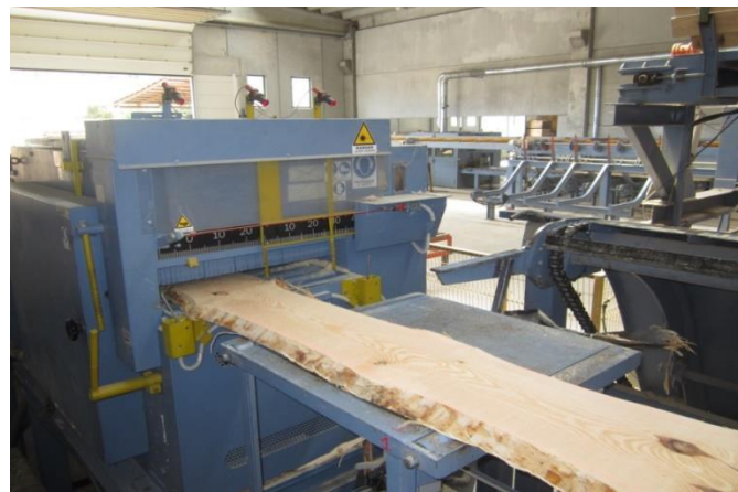
Figure 5 - Example of multi blade cutting
