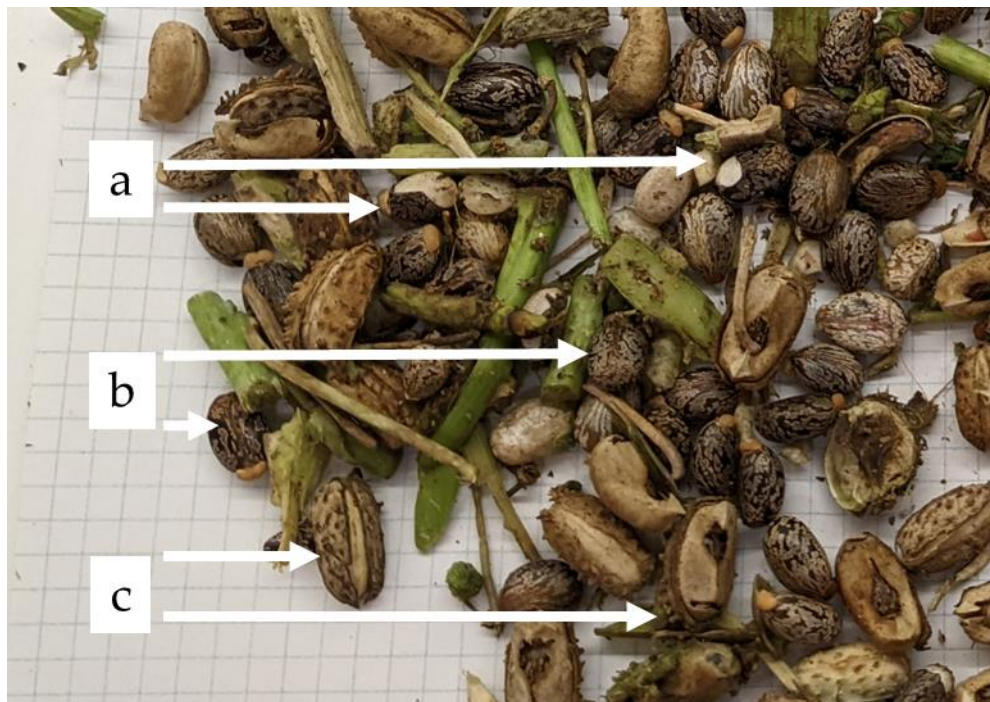
Figure 6. Sample of seeds collected within the tank of the combine harvester showing: a) damaged seeds; b) undamaged seeds; c) unopened seeds.
