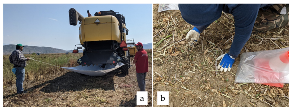
Figure 3. Collection of threshed biomass (a) and lost capsule (b) for CSL and ISL assessment, respectively.
