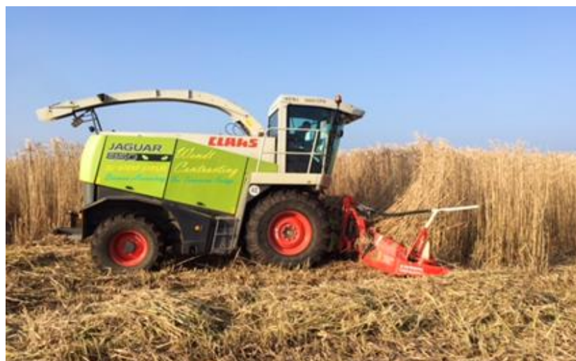
Figure 2. Miscanthus harvesting in a single pass using a self-propelled forage harvester.
