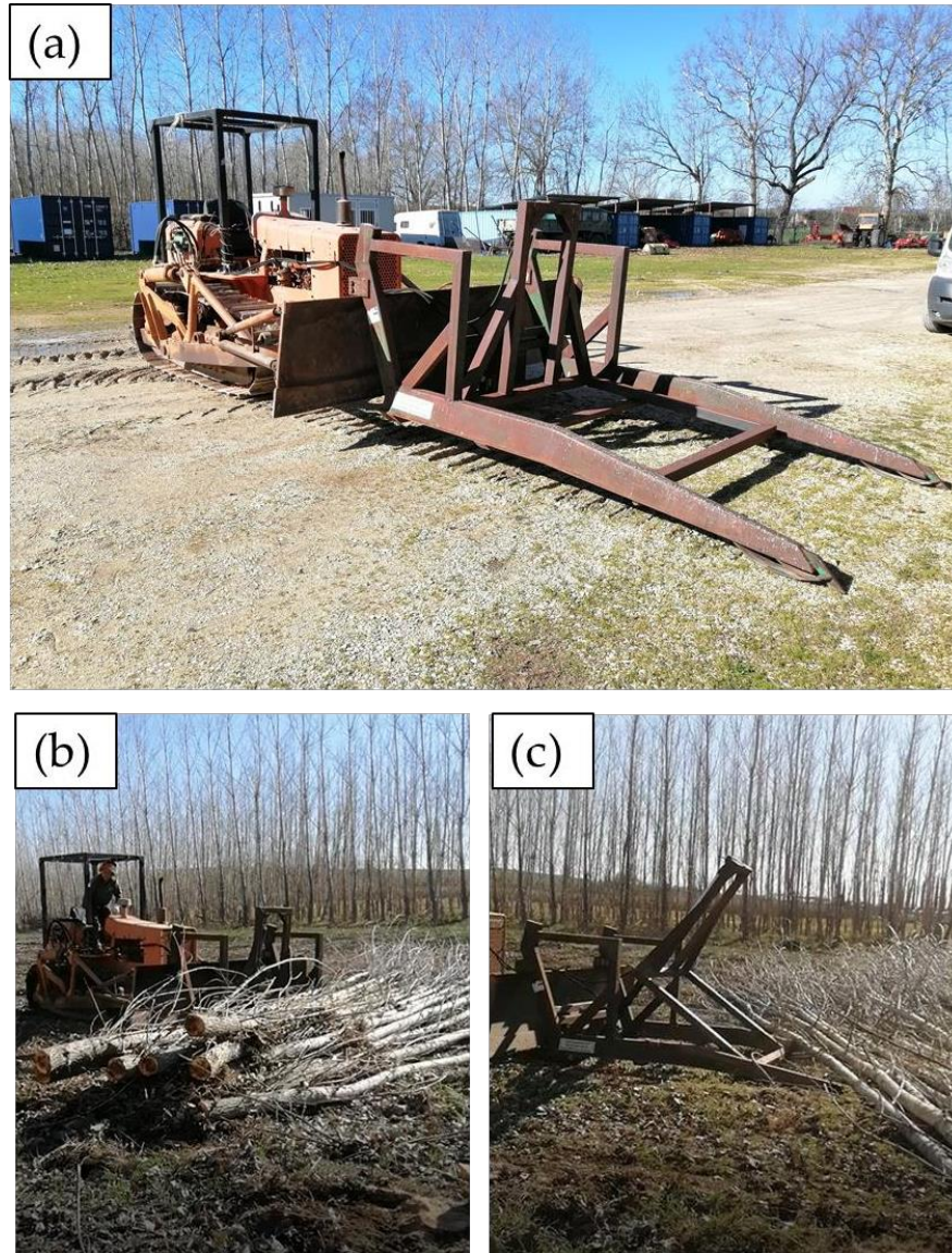
Figure 14. (a) Vision of CFL. (b) CFL while loading trees. (c) CFL while unloading trees.
