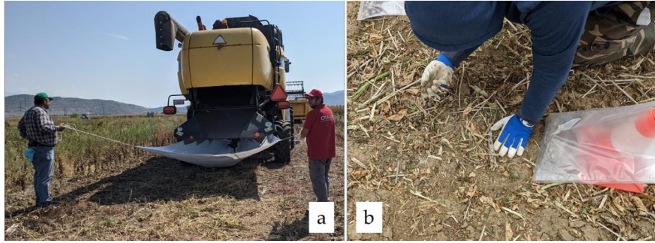
Figure 5. Collection of threshed biomasses (a) and lost capsule (B) for CSL and ISL assessment respectively.
