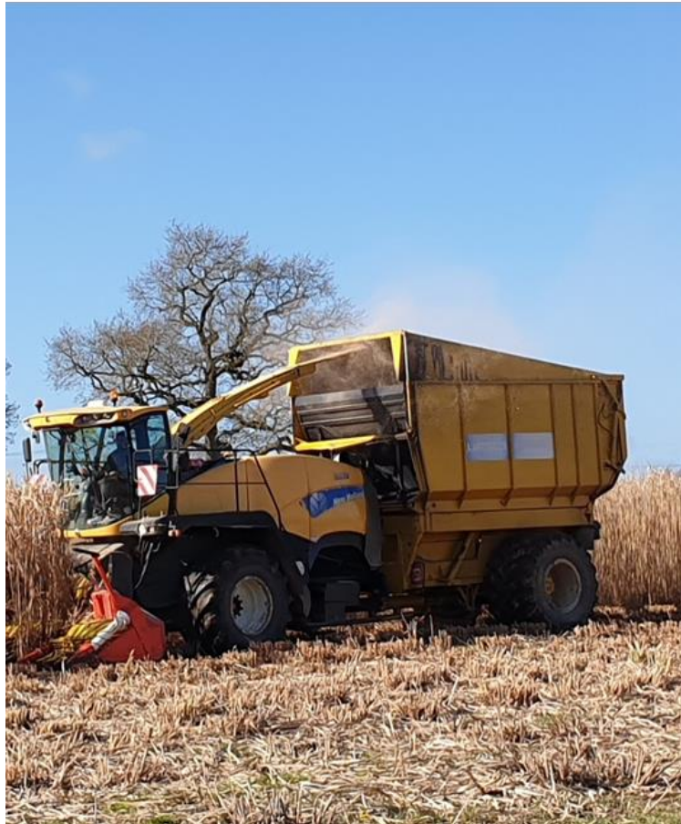
Figure 3. Miscanthus harvesting by self-propelled forage harvester.
