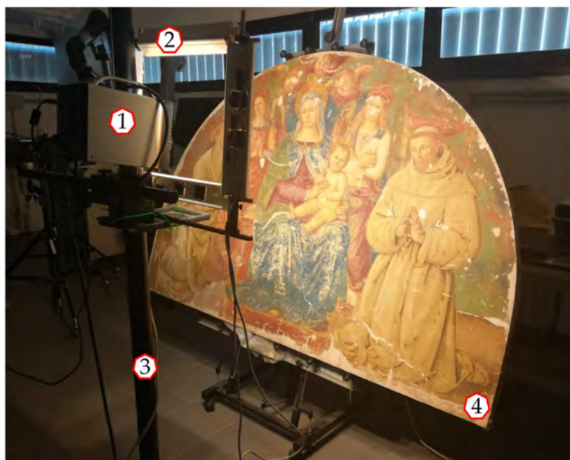
Figure 3. PuCT experimental setup: (1) Thermal camera; (2) rectangular plastic frame, which houses two LED chips per side; (3) tripod; (4) inspected wall painting lunette.
