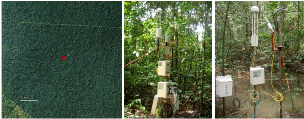
Figure 3.1. Left panel: aerial image of the below canopy measurement site (white triangle) showing its proximity to the main tower (red square). The middle panel shoe the system set-up for April (in the dry season) and the panel on the right the set-up for October (wet season). Note the difference in the soil water content below the instruments: in October there was a water layer of about 20 cm thickness.
