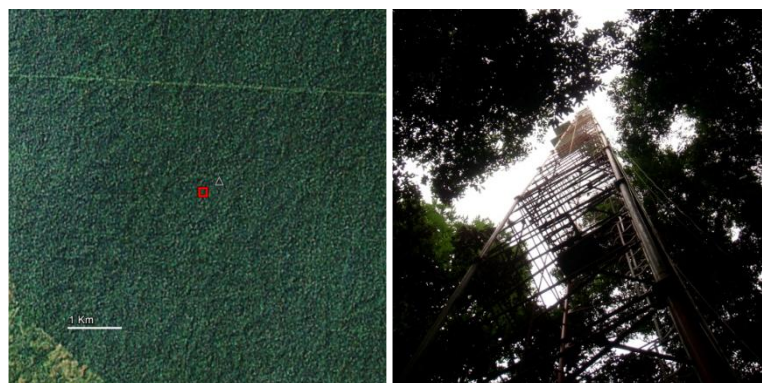
Figure 4.1. Left panel: aerial image of the main tower (red square) location. Right panel: a perspective from the tower base. The storage system air inlets are placed on the north side of the tower structure at 0.4, 0.8, 8.5, 18, 24, 48.9 and 64 m from the soil.
