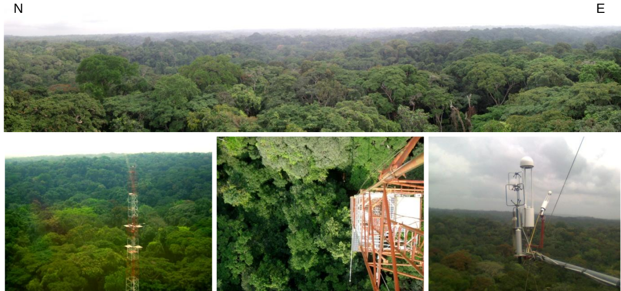
Figure 5.1. Outlooks of the Ankasa EC tower station. At the top, a panorama from the tower spanning from north to east. At the bottom from the left an aerial picture of the tower, a view from the tower top and a particular of the measuring sensors (note that the second anemometer is part of a concurrent measurement system)
