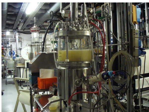
Figure 11: 20-L bioreactor for producing P. phosphoreum on industrial scale (a) and continuous greenish-light, coming from the cultivated light-emitting bacteria (b)
