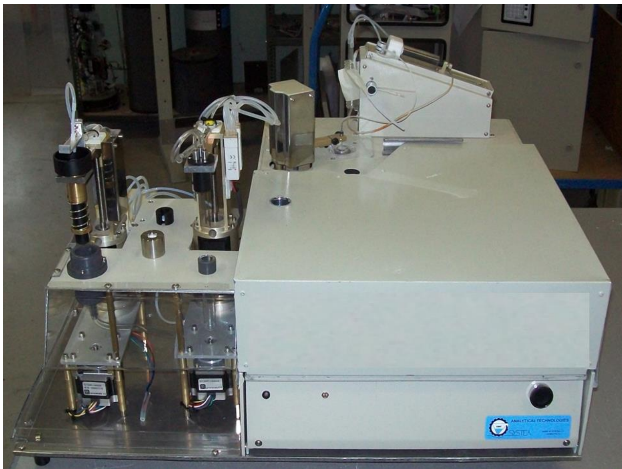
Figure 30: Final assembling of Easy coli analyser, consisting of the filtration unit in the left part and the detection unit in the right.
