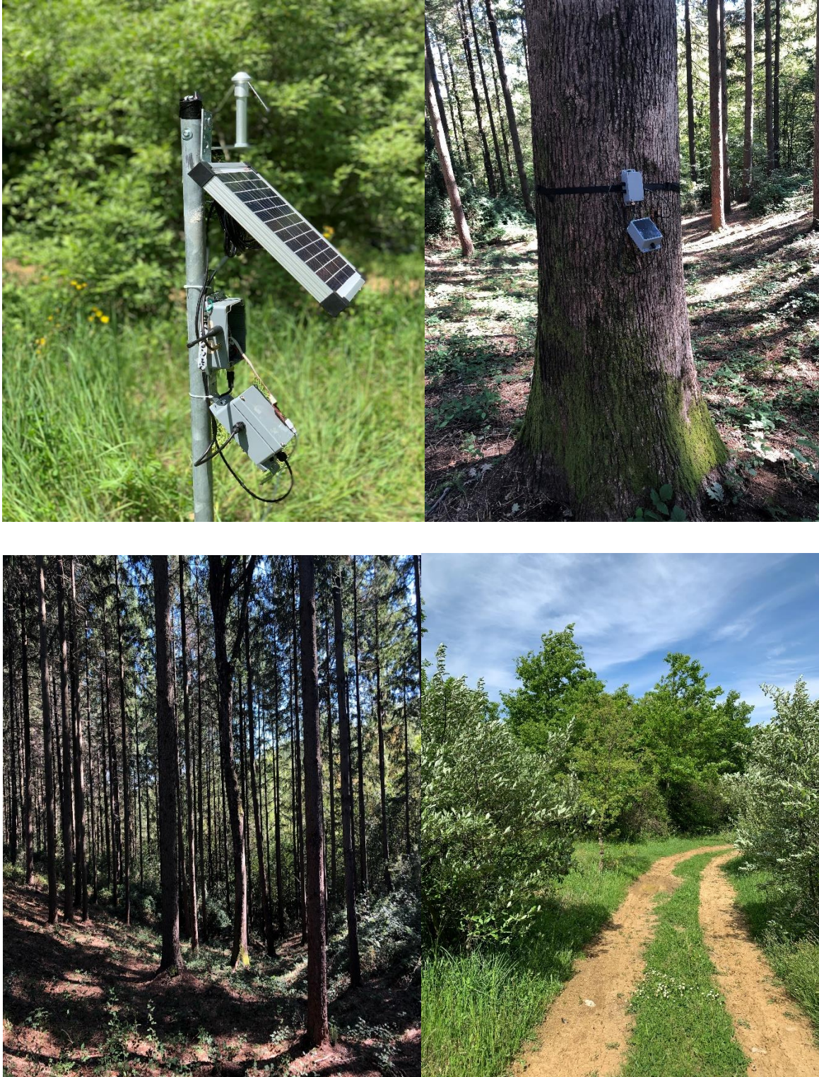
Appendix. 6: Top 2 (Left to right) pictures showing TT Cloud with antenna and solar panel and Tree talker device installed on Quercus petraea L. Bottom 2 (left to right) pictures showing site 1 and site 2.
