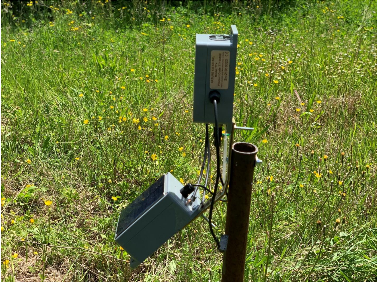
Fig. 6. Tree Talker with solar panel attached to the battery pack, without tree to obtain direct light transmission.
