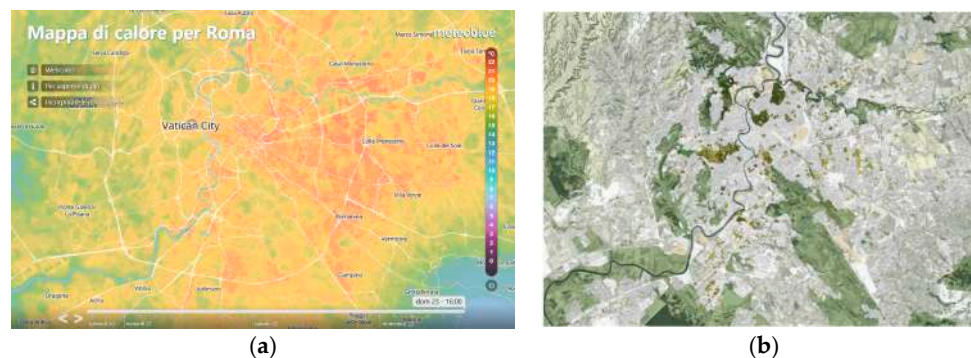
Figure 2. (a) Real-time mapping of the urban heat island in Rome. It can be seen that the most critical areas (orange-red color) are located in the eastern part of the city, while in the western part, the presence of vegetation has a mitigating effect that lowers the urban temperature. (b) Mapping of green areas in Rome.
