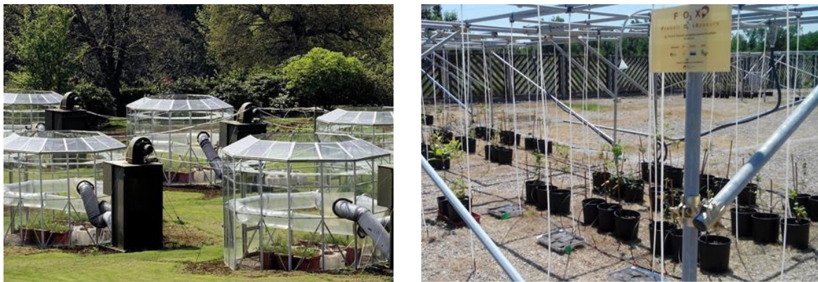
Figure 4 - Two examples of structure for manipulative experiments. On the left: Open Top Chambers (OTCs), Newcastle University (UK) Close House field station (Simon Fraser©). On the right: Free Air Concentration Enrichment facility (FACE), National Research Center (CNR), Sesto Fiorentino (Italy).
