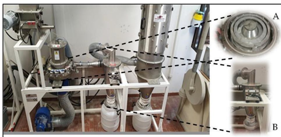
Figure 2. Micronizer pilot plant improved through the addition of a grinding chamber including a hammer crusher impeller (A) and a decanting collector (B).
