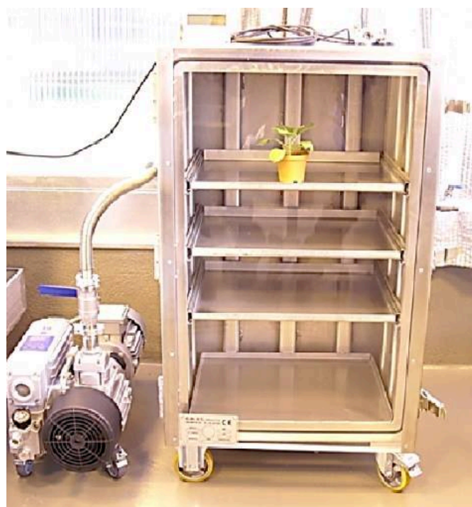
Figure 3: Vacuum chamber used at laboratory scale for transient plants transformation.
