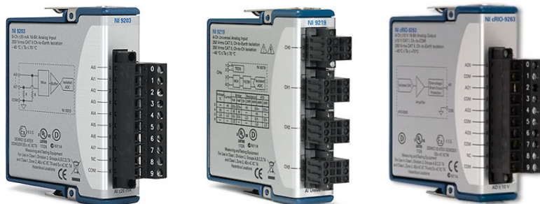
(a) NI 9203: input current (n.8 channels, \pm 20 mA, 16-bit resolution). (b) NI 9219: input current ( \pm 20 mA) or voltage ( \pm 60 V). (c) NI 9263: analog voltage output (n.8 channels, 0-10 V, 16-bit resolution, 100 kS/s).
