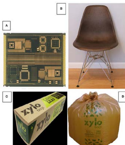
Figure 1.10 Semi-commercial products with lignin—(A) Prototype printed circuit board manufactured with glass fiber-reinforced (organosolv) lignin-containing (50%) epoxy resin (B) Prototype shell of injection-molded chair made from polypropylene/lignin derivative blend; and (C,D) commercial compostable waste bag made with melt-blown films of blends of hydroxypropyl (Kraft) lignin derivative and biodegradable polyester. 74
