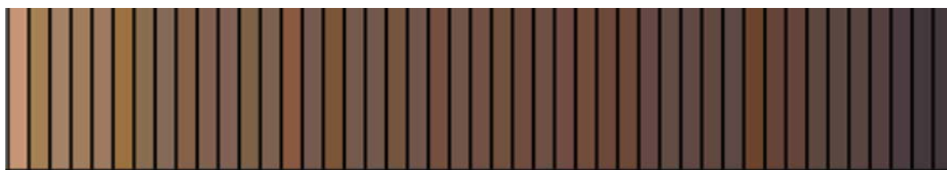
Figure 1.7 Colour of 45 lignin samples arranged in order of decreasing brightness
