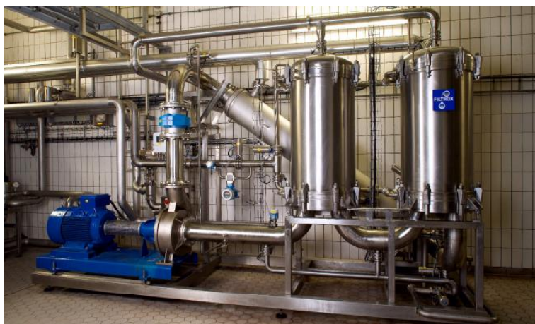
Figure 1.27 Anisotropic ceramic CFMF membrane unit.
