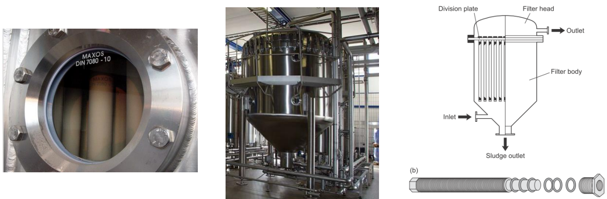
Figure 1.19: Schematic views of vertical (a) and horizontal leaf filters (b) .
