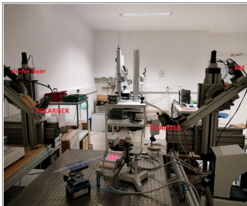
Figure 48. Overview of the experimental ellipsometer setup (available at IPR, Rennes, France): a He-Ne laser ( \lambda = 633 nm) is linearly polarised, reflected by the Langmuir trough surface, and becomes elliptically polarised. A quarter-wave plate and rotating analyzer convert and extinguish the beam, with intensity detected by a photomultiplier (PM).
