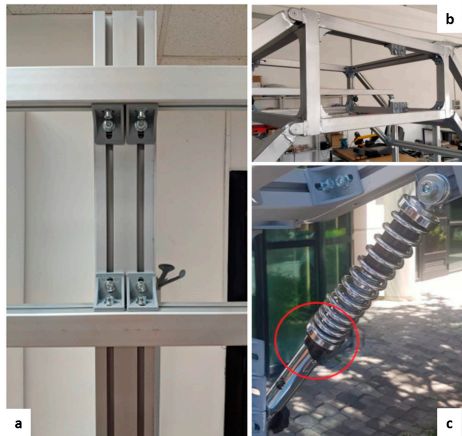
Figure 2. (a) Vertical seat for instrumentation; (b) crossbar with knobs for track adjustment; (c) ring nut for shock absorber preload.
