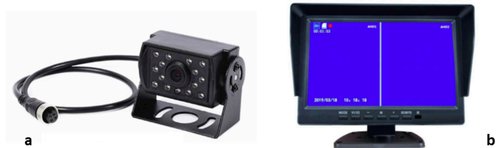
Figure 9. (a) Video camera; (b) 10.1" IPS 1024*600 resolution screen.
