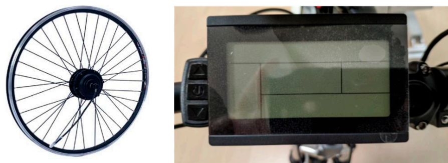
Figure 5. Motorized wheel (on the left); display and motor start button integrated in the wheel (on the right).
