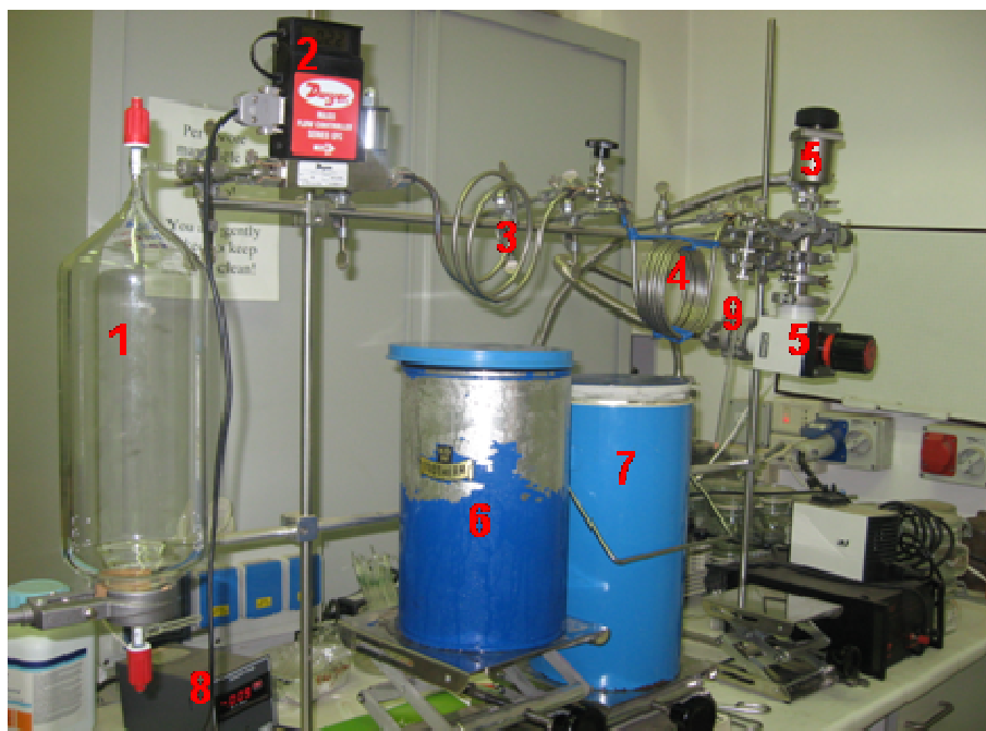
Fig. 4 Cryogenic line: 1-sample 2L flask with CO 2 , 2-mass flow meter and controller; 3-H 2 O trap; 4-CO 2 trap; 5-pumping system; 6-dry ice ethanol mixture; 7-liquid mixture; 8-pressure gauge; 9-test tubes
