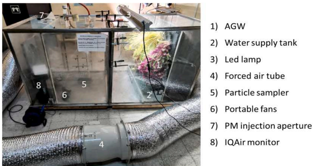
Fig. 2. Closed glass chamber for experiments with active green wall (AGW).
