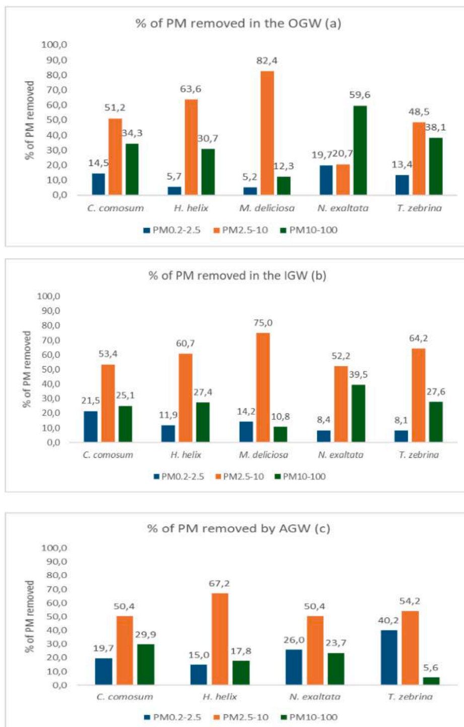
Fig. 5. PM accumulation percentage on plant species in outdoor green wall (OGW), indoor green wall (IGW) and active green wall (AGW), per size fraction.
