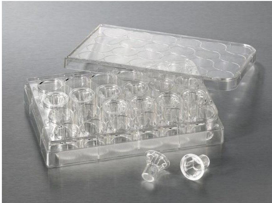
Figure 1 - 24-well plate with transwell inserts for air-liquid interface cell culturing
