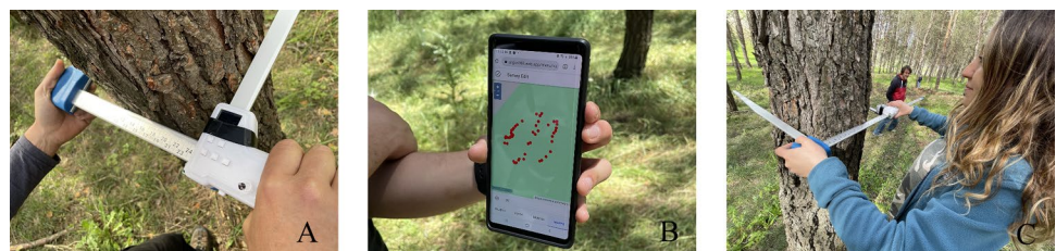
Fig. 2 Hardware and software use-case; A detail of the complete prototype; B Detail of the web-app, GPS tagging section; C Operator testing the tool
