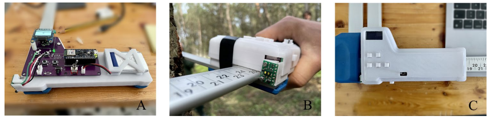
Fig. 1 A prototype of IoT open-source digital forest caliper: A PCB and electronics design exposed; B placement of the time-of-flight sensor; C buttons placement and overall shape
