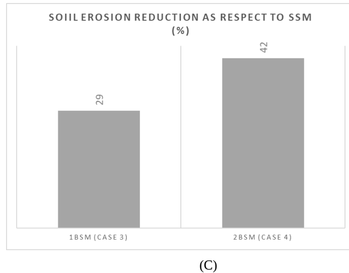
Figure 2.5. (A) Annual soil erosion; (B) percentage increases of soil erosion for cases 2-3-4 as respect to case 1 (intact forest); (C) percentage decreases of soil erosion for cases 3-4 as respect to case 2 (SSM).
