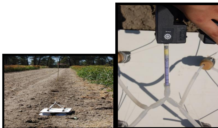
Fig 2.4. Chamber method for determining ammonia in the field – (Drager-Tube Method, DTM)
