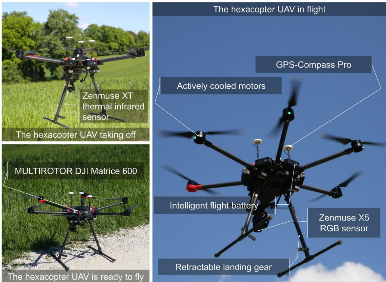
Supplementary figure 4.1 The DJI Matrice 600 unmanned aerial vehicle (UAV) platform used for field phenotyping of Triticum turgidum (cv. Marco Aurelio) on the ground, taking off, and in flight.
