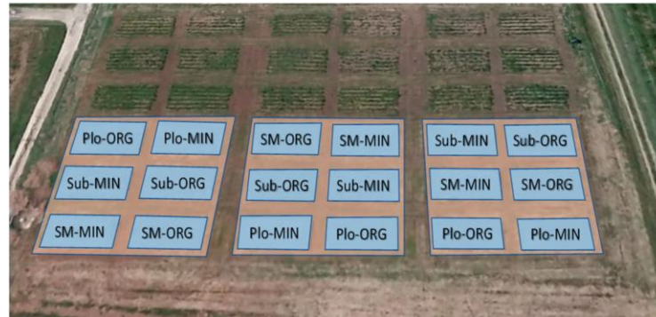
Figure 1. Experimental field plan in the 2013/2014 growing season of durum wheat. MIN = mineral fertilization; MOW = municipal organic waste; Plo = plowing; Sub = subsoiling; SM = spading machine.
