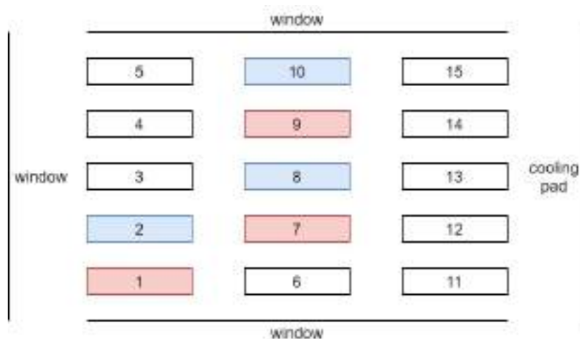
Figure 4. Experimental units in the greenhouse under two different lighting treatments in the first experiment. Plants on the pink benches were grown using the prediction-based lighting method, and those on the blue benches were grown using the heuristic method.
