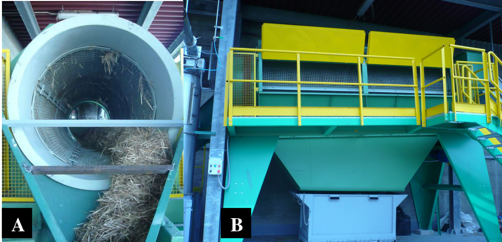
Fig.10 Rotating grid during operation (A) and lateral view (B).
