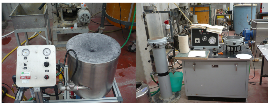
Fig.31 Laboratory scale flotation de-inking cell during operation (left) and standard Rapid Koethen paper sheets preparation equipment (right).
