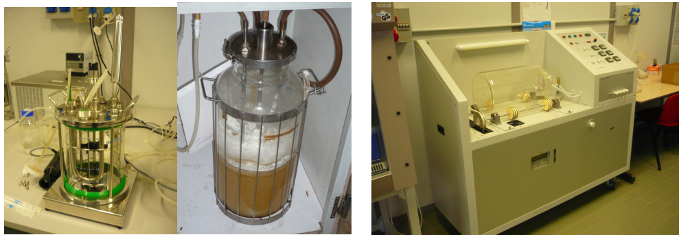
Fig.24 2.5 l laboratory scale liquid fermenter (left); 25 l liquid fermenter (middle) laboratory scale SSF fermenter (right).
