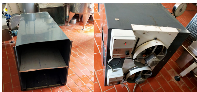
Figure 4. Dehydration tunnel (front) with the two fans (back) used in the laboratory experiment.
