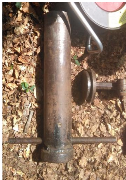
Fig. 10 A steel cylinder core tube used for sampling
