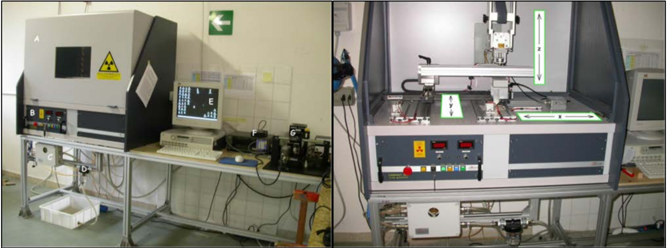
Figure 14. X-ray densitometer, for wood density analyses, located at Italian National Research Council – Trees and Timber Institute, in S. Michele all’Adige (TN, Italy).
