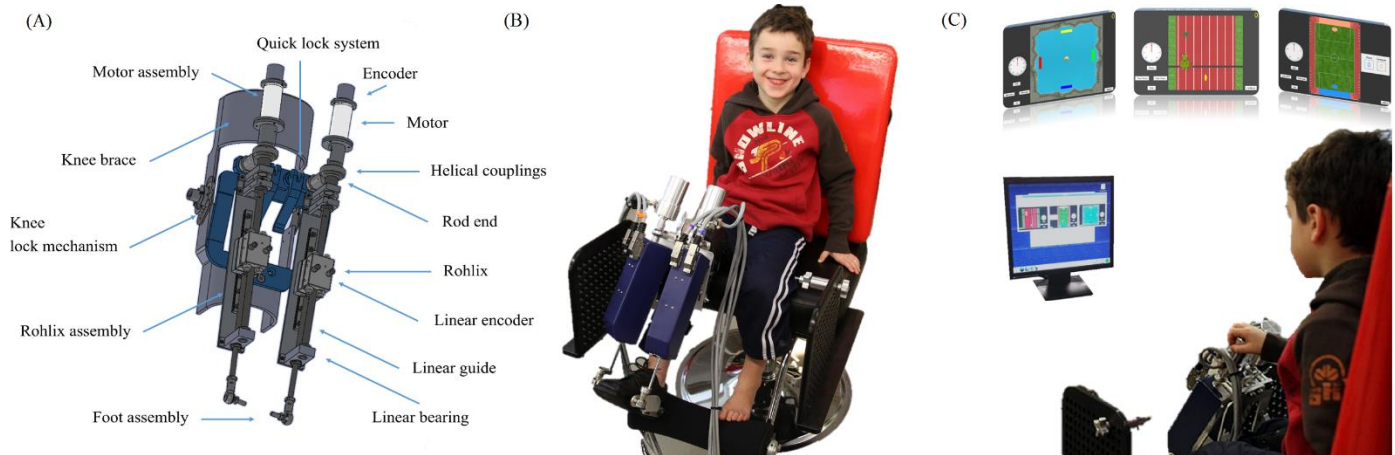
Fig. 1. The MIT's pediatric ankle robotic system (pediAnklebot). (A) The mechanical design of the robotic prototype showing the components of the device (B) A 7-year old child wearing the pediAnklebot in seated position; the weight of the pediAnklebot is supported from the chair, through a bolt (C) playing the serious games that were developed for the device based on motor learning principles in a 20" screen positioned 1 m away from the kid (clinical setup).
