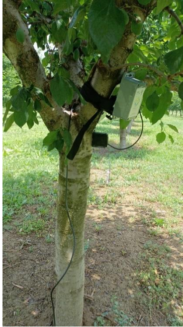
Figure 13: Tree Talker device monitoring radial stem growth.
