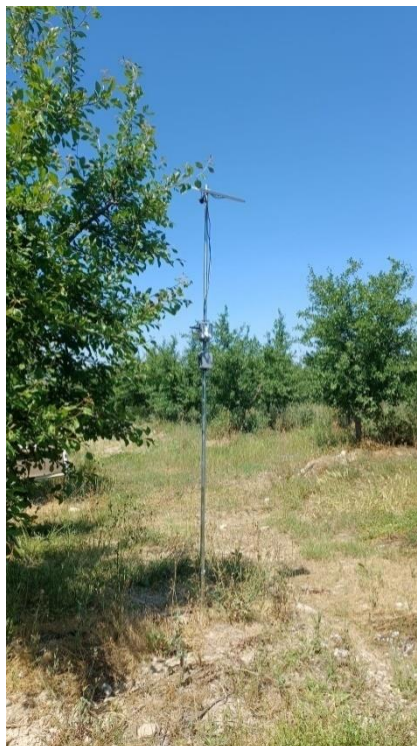
Figure 14: Wireless station receiving the data from the Tree Talkers and sending them via GSM to central server.
