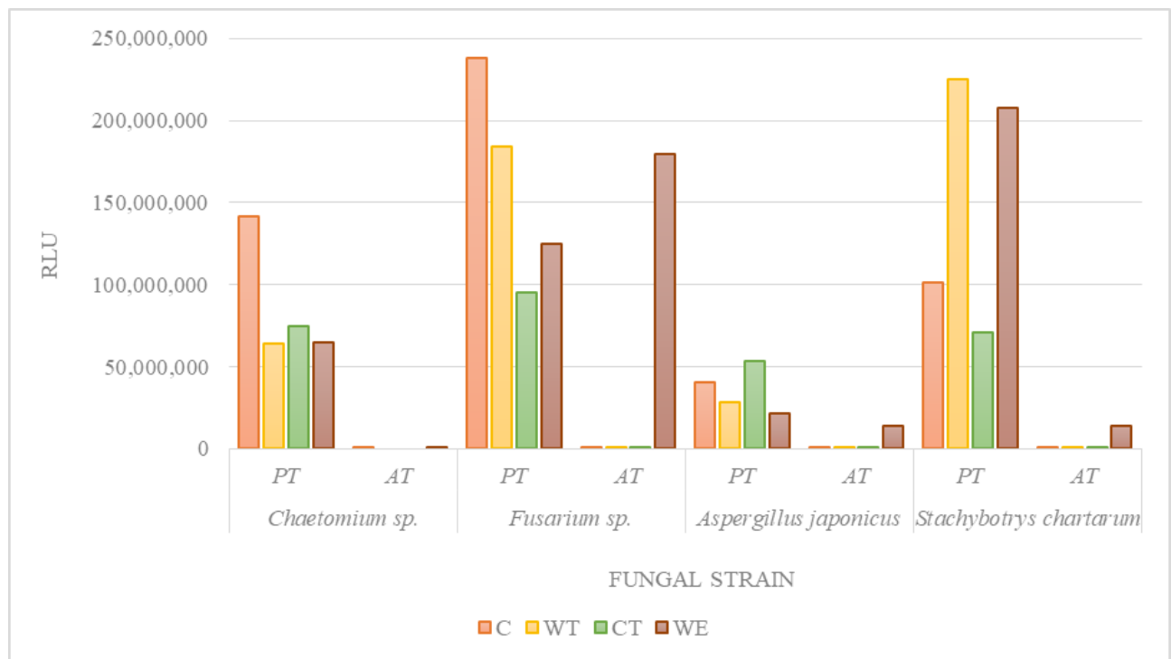
Figure 23. Evaluation through ATP bioluminescence assay of the biocidal activity of cinnamon (C), wild thyme (WT) and common thyme (CT) oils MIC against mycelium of Chaetomium sp., Fusarium sp., Aspergillus japonicus and Stachybotrys chartarum . Control tests were performed treating the mycelium with a solution of deionised water and ethanol (WE). (PT: pre-treatment, AT: after treatment).
