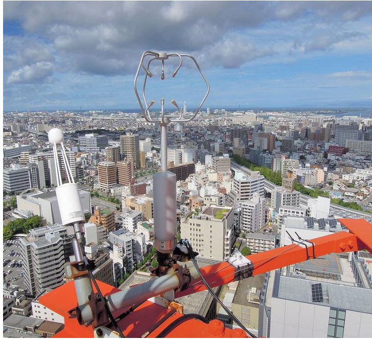
Figure 2. EC site accessorized with gas analyzer on the left side and sonic anemometer on the right-side at Sakai city office, Sakai, Japan
