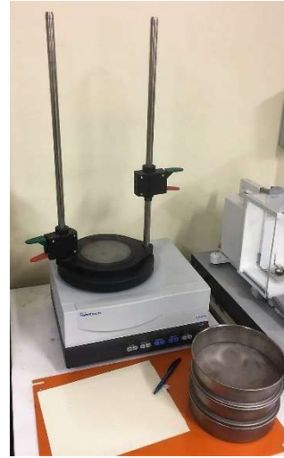
(b) vibratory sieve AS 200 Control
