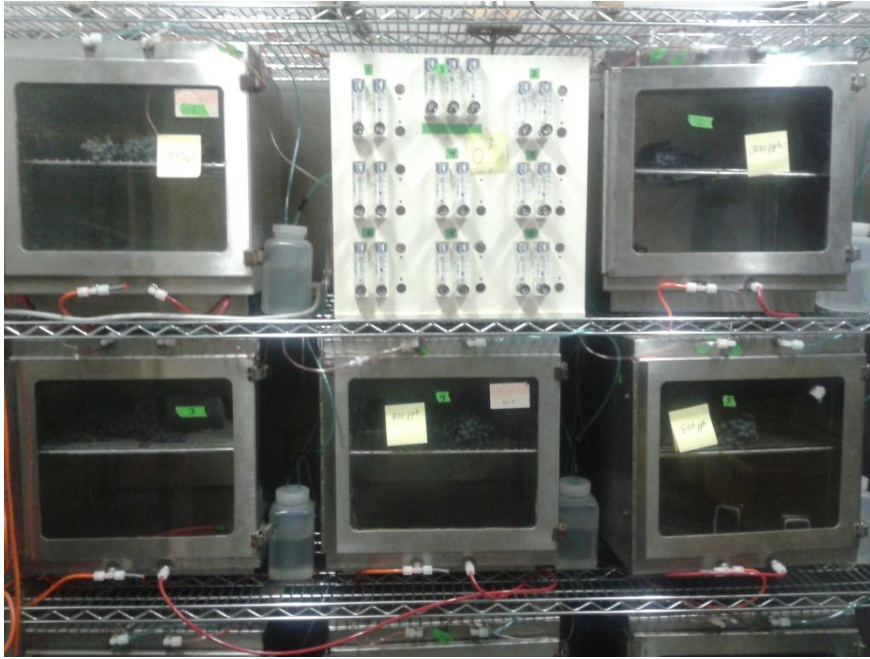
Fig. 4.1.2 Thermohygrometric cells for multiples ozone concentration treatments.
