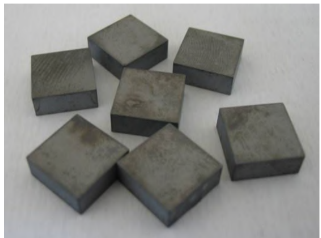
Fig. 1 WC–Co specimens used for the experiments
