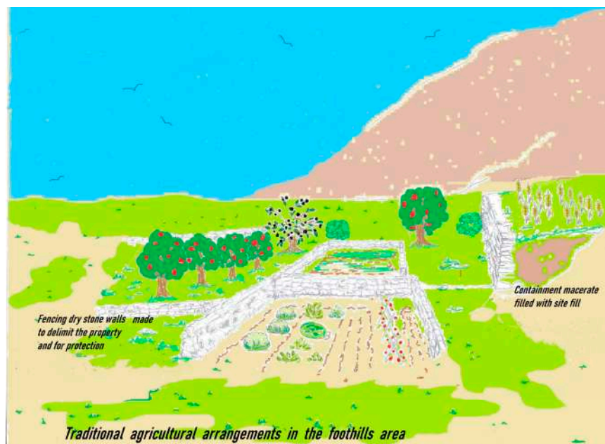
Figure 5. Schematic representation of the utilization of dry-stone walls for safeguarding crops from grazing animals, delineating property boundaries, and mitigating hydrogeological disturbances.
