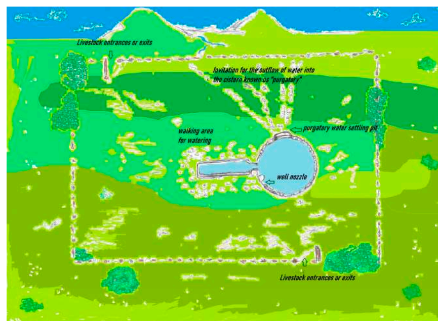
Figure 4. Schematic depiction of a traditional water reservoir and watering system.
