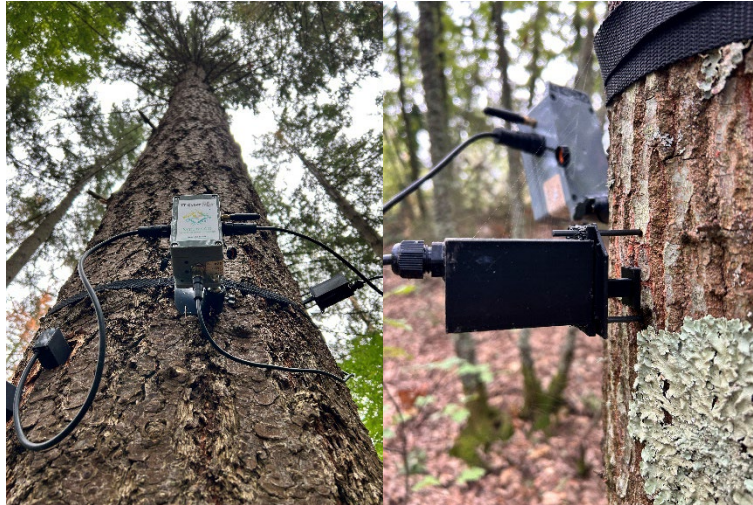
Figure 2: Installation of Treetalker with LME dendrometer installed on a P. Abies with several other measuring systems.
